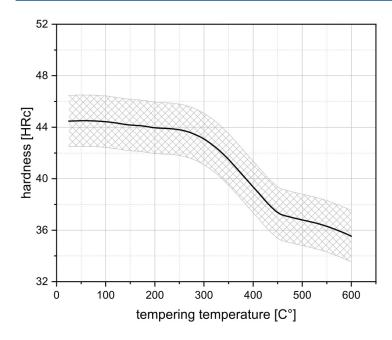
Heat treatment Hardening temperature 850°C Soaking time 30 min water quenched
