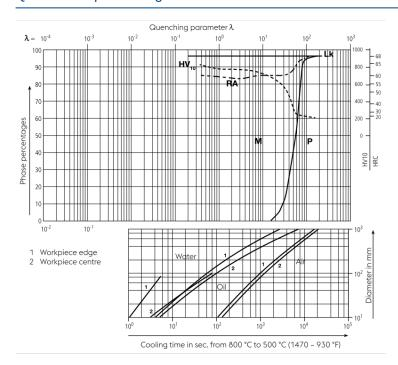
O Vickers hardness LK... Ledeburitic carbides RA... Retained austenite M... Martensite
