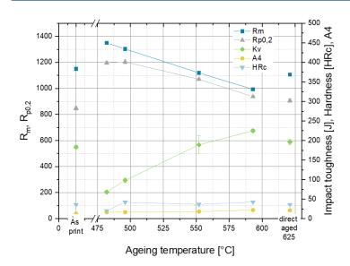
Solution annealing: 1040°C / 30min / air quenching
