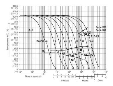
Austenitising temperature:  $1025^{\circ}$ C ( $1877^{\circ}$ F) Holding time: 15 minutes 5...100 phase percentages 0.5...180 cooling parameter, i.e. duration of cooling from  $800 - 500^{\circ}$ C ( $1472-932^{\circ}$ F) in s x  $10^{-2}$
