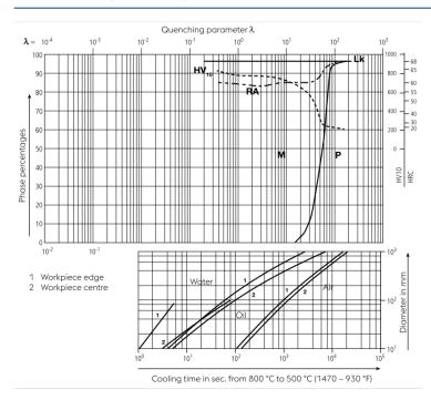
O Vickers hardness LK... Ledeburitic carbides RA... Retained austenite M... Martensite P... Perlite
